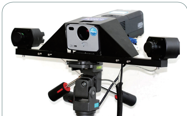
Figure 1 Structured-light 3D scanner. It consists of two charge-coupled device cameras and one projector.
